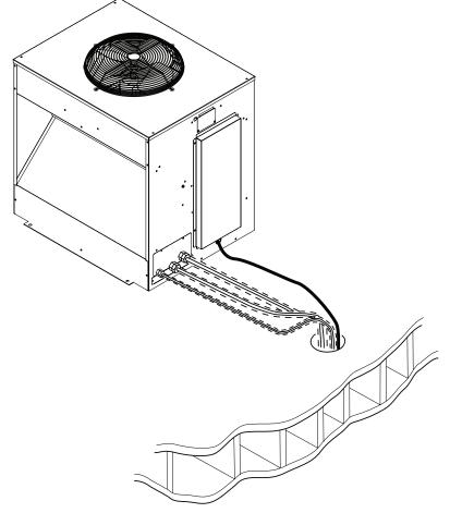
The line set must be routed between the condensing unit and the ice maker's location. During the transition from quick connects to braze connections, the ice maker, condensing unit and line set may or may not have quick connects, use this chart as a guideline for the proper action based on what is available at the site.
