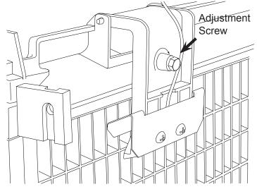
Bridge Thickness Adjustment Mechanism
